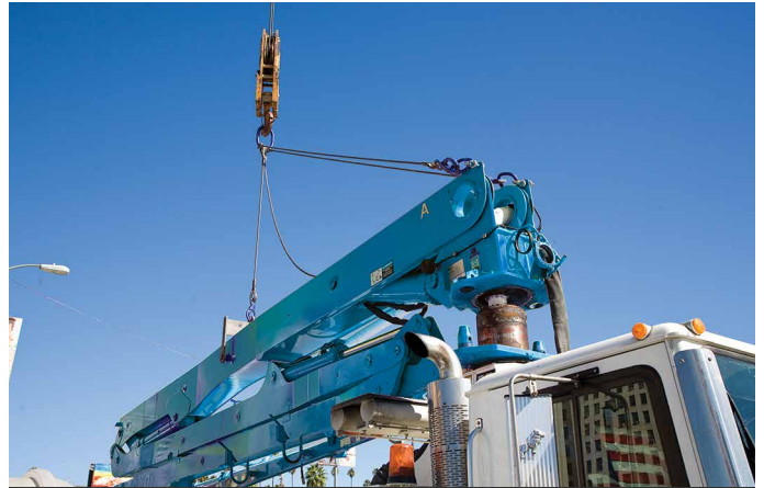
STEP 2 – Detach boom and lift
