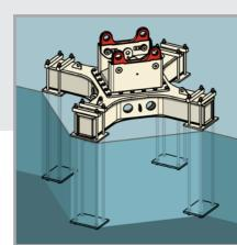
Attached on a base plate with anchors embedded in the foundation <sup>(2)</sup>
