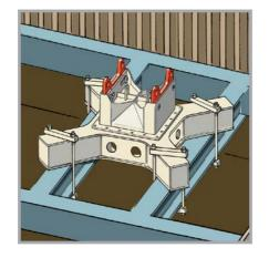
Cruciform base mounted on a shaft frame with tie-rods <sup>(6)</sup>
