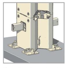
RS-850 with existing base plate and slab fixed with four base plates <sup>(4)</sup>
