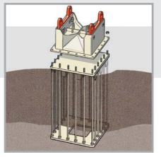
Compact cruciform base anchored in the foundation with a tie-rod cage (when space is restricted) <sup>(3)</sup>
